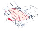
**4** Press release buttons on each hook and push hook into larger tube.
